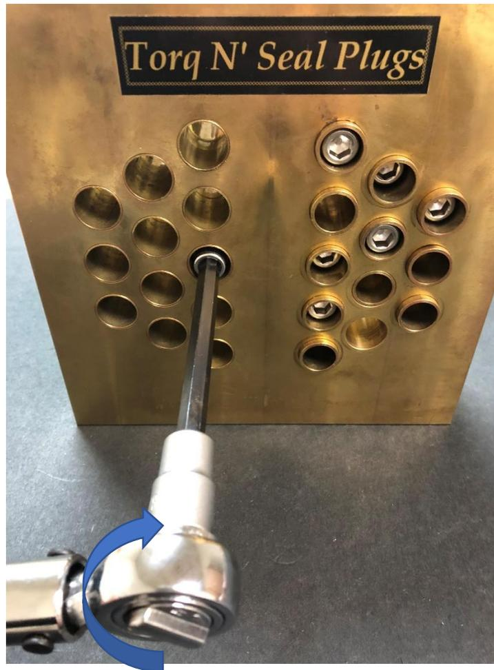
Remove the Hex Capture Drive from the plug with a swift pull away from the tubesheet and installation is complete. Your tube is now sealed in excess of **6,500 psi** by Torq N' Seal®, simple as that.
