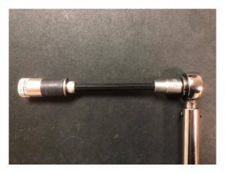
**Set your torque wrench to 120 in-lb**. Align the cam with the plug body and insert the plug into one end of the leaking tube. Insert the plug until the rubber portion is all the way into the tube, this will ensure maximum sealing area on the tube Inner Diameter and a confident seal.
