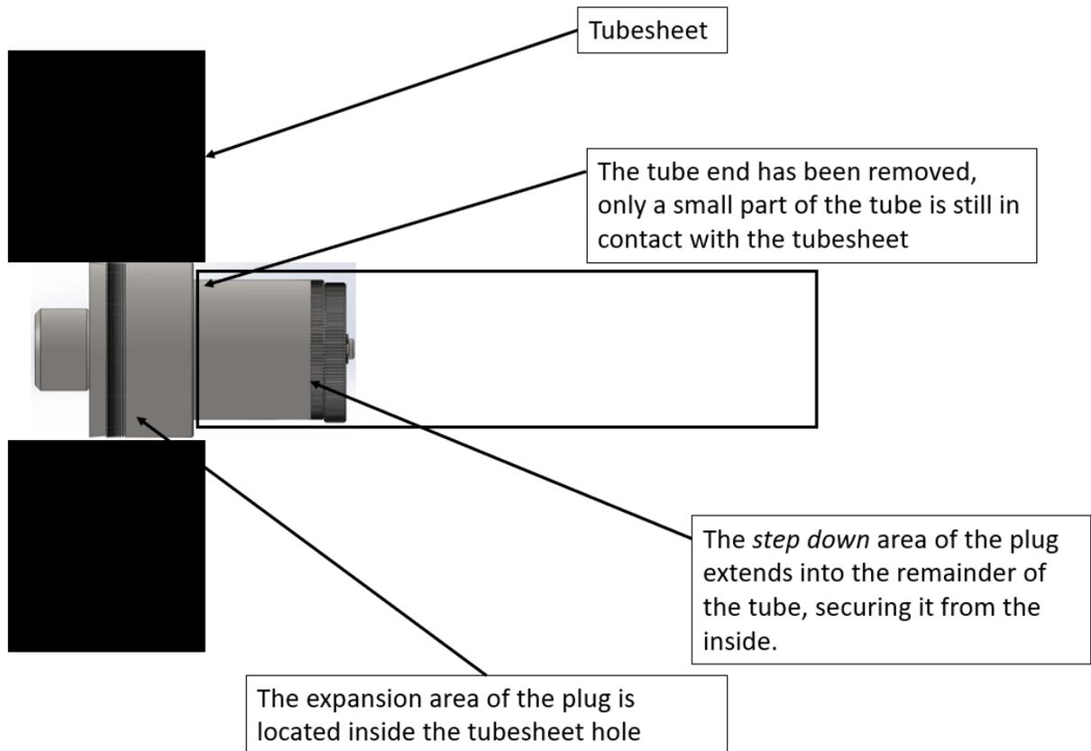
The *step down* area of the plug is designed to fit within the remainder of the tube. Meanwhile, the expansion area is large enough to plug the tubesheet hole directly, where the tube end has been
